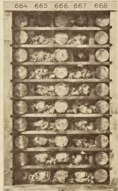
Cylinders of different brands of standard Portland cement cured in distilled water 20 days, after three years in lake
